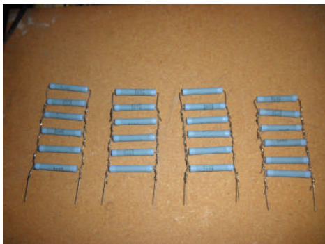
I assembled the resistors into four 200-ohm loads
