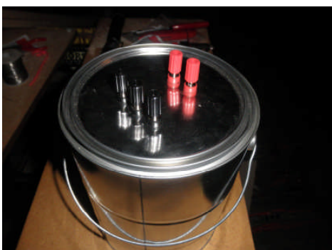
This allows the load to be configured for 50 \Omega , 100 \Omega , 200 \Omega , 300 \Omega , 400 \Omega , 600 \Omega and 800 \Omega .
